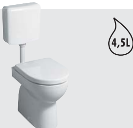
Renova Nr. 1 wash-down WC, 4,5 l/6 l, floor-standing, free inlet, vertical internal outlet, 355 x 875 x 675 mm, Model-no. 213011. Combinable with plastic cistern 4,5 l/6 l, Model-no. 521031. WC seat Renova Nr. 1 Plan: Model-no. 573075. Model-no. 573085 with soft closing mechanism.
