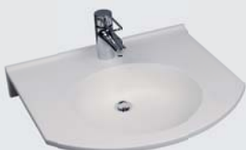
Privo wash basin made from Varicor®, without overflow, wheelchair-accessible, DIN 18040, 600 x 550 mm, model no. 402060 without cut-outs.
