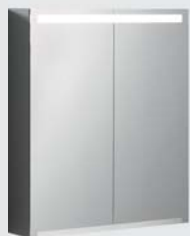
Cabinet with mirror , with integrated LED-light, washbasin light, 2 doors mirrored on both sides, 2 adjustable glass shelves, 1 electric socket, 1 light-touch-sensor-switch. Max. 14,95 Watt, 230 V, 50 Hz, 4100 K, 1020 lm (above)/935 lumen (below), IP44, safety class 2, energy class A++, 600 x 700 x 150 mm, Model-no. 800360.
