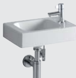
Hand-rinse basin, without overflow, 380 x 280 mm. Model-no. 124836 with tap hole left. Model-no. 124736 with tap hole right. With shaft valve with domed cover cap. Combinable with vanity units for hand-rinse basins 370 mm.
