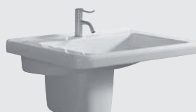
Washbasin, with tap hole, without overflow, accessible by wheelchair, DIN 18040, two levels for water inside, 600 x 550 mm, Model-no. 128662. Combinable with half-pedestal, Model-no. 298510 or washbasin vanity units 530 mm.
