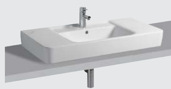
Renova Nr. 1 Plan countertop washbasin, with tap hole, with overflow, 1000 x 480 mm, Model-no. 125100. For wall-mounting.
