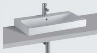
iCon countertop washbasin, with tap hole, with overflow, 750 x 485 mm, Model-no. 124575. For wall-mounting.
