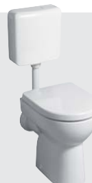
Renova Nr. 1 wash-out WC, 6 l, floor-standing, free inlet, horizontal outlet, 355 x 875 x 705 mm, Model-no. 203010. Combinable with plastic cistern 4,5 l/6 l, Model-no. 521031. WC seat Renova Nr. 1 Plan: Model-no. 573075. Model-no. 573085 with soft closing mechanism.
