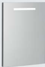
Illuminated mirror element with switch, T5/8W, 6400 K/260 lm, 230 V, ~50 Hz, IP 44, safety class 2, energy class A+, 500 x 650 x 35 mm, model-no. 862350.
