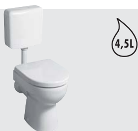
Renova Nr. 1 wash-down WC, 4,5 l/6 l, floor-standing, free inlet, horizontal outlet, 355 x 875 x 705 mm, Model-no. 213010. Combinable with plastic cistern 4,5 l/6 l, Model-no. 521031. WC seat Renova Nr. 1 Plan: Model-no. 573075. Model-no. 573085 with soft closing mechanism.
