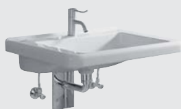
Washbasin, with tap hole, without overflow, accessible by wheelchair, DIN 18024 part 2, DIN 18025 part 1+2, two levels for water inside, 550 x 525 mm, Model-no. 128557. Combinable with half-pedestal, Model-no. 298510.
