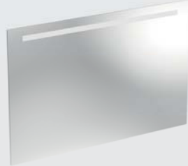
Illuminated mirror element , with integrated switch, T5, 21 W, 4000 K, 230 V, ~50 Hz, IP 44, safety class 2, energy class A, 1000 x 650 x 36 mm, Model-no. 800400.
