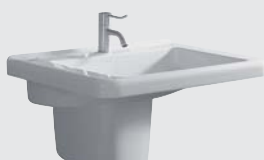
Washbasin, with tap hole, without overflow, accessible by wheelchair, DIN 18024 part 2, DIN 18025 part 1+2, two levels for water inside, 550 x 525 mm, Model-no. 128557. Combinable with half-pedestal, Model-no. 298510.
