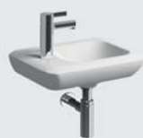
Hand-rinse basin, without overflow, 400 x 280 mm. Model-no. 272940 tap hole left. Model-no. 271940 tap hole right. Shaft valve with domed cover cap. Combinable with hand-rinse basin vanity units 304 mm.
