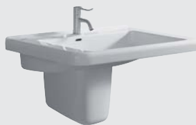
Washbasin, with tap hole, with overflow, accessible by wheelchair, DIN 18040, two levels for water inside, 600 x 550 mm, Model-no. 128660. Combinable with half-pedestal, Model-no. 298510 or washbasin vanity units 530 mm.
