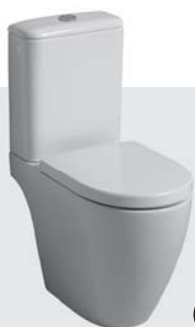
Wash-down WC combination, rimfree, 6 l, floor-standing, outlet Multi, 375 x 830 x 640 mm, Model-no. 203400. Ceramic cistern with dual flush 3 l/6 l, Model-no. 229420. WC seat, Model-no. 574120. WC seat with soft closing mechanism, Model-no. 574130.
