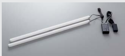
LED-strip lights , 4000 K, IP21, energy class A++, for universal use. 440 mm, (1 pair), max. 2 x 4 W, 896 lm, Model-no. 501470. 550 mm, (1 pair), max. 2 x 4,75 W, 1064 lm, Model-no. 501550. (Please pay attention to the power connection.)
